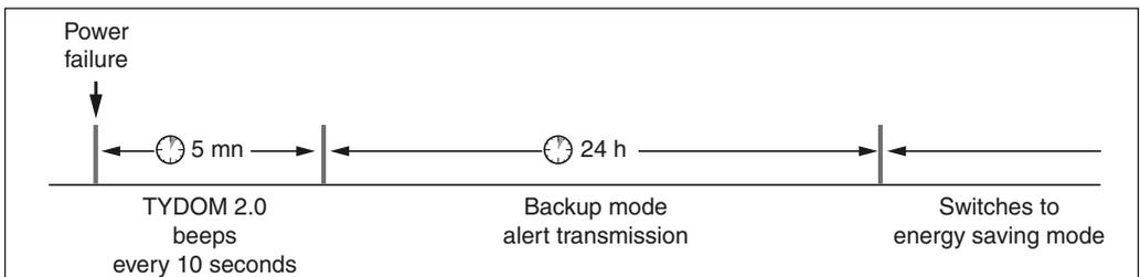
During a power failure, the video transfer function is not available. The transfer of video links will resume when the power and Internet access are restored.
