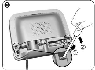
Using a screwdriver, lift the 2 clips holding the top cover.
