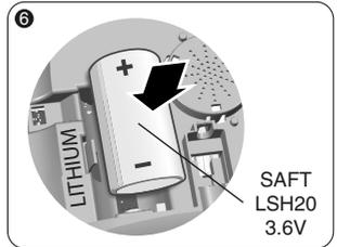
Insert the battery, observing the right polarity.
